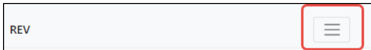
Figure 9: Module Navigation is collapsed when narrow, with bento box icon at right which when clicked shows all module top navigation
